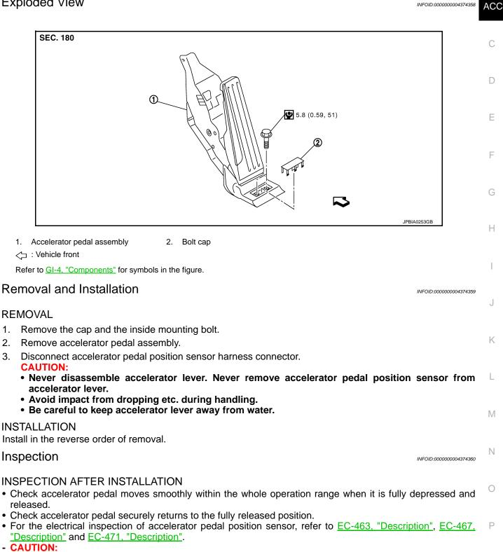
When harness connector of accelerator pedal position sensor is disconnected, perform "Accelerator Pedal Released Position Learning". Refer to EC-18, "ACCELERATOR PEDAL RELEASED POSITION **LEARNING : Description".**
